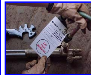
Employee inspecting and confirming torch end ID number matches supply end.
